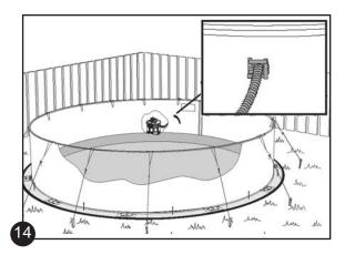
Tape the end of the vacuum hose before inserting it into the wall so as not to damage the liner.
