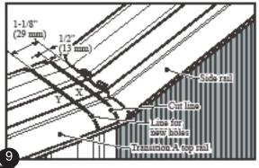
along to shorten the transition rail. The seconde line Y is also parallel to the end of the side rail, 1-1/8" (29mm) away, this will be the line that the new 1/4" (6mm) screw holes lie on.
