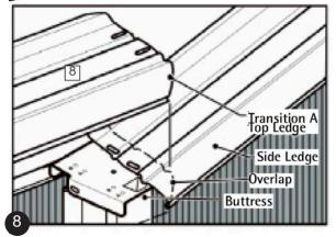
c. With the end of the side rail on top of the transition rail, mark two dimension 1/2" (13mm) and 1-1/8" (29mm) away from the end of the side rail. Then temporarily unscrew the other end of the side rail and move it to draw the lines X and Y. The first line **X** is parallel to the end of the side rail, 1/2" (13mm) away. This will be the line you will cut
