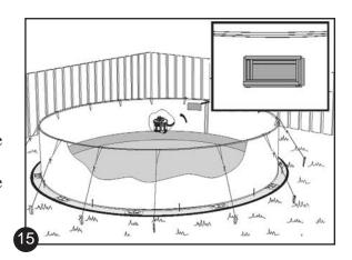
f. Close the skimmer opening with cardboard and adhesive tape so that the suction of air works better..
