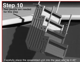
Carefully place the assembled unit into the pool and tip it  $45^\circ$  to the left, right and forward to fill steps with water. Repeat if steps continue to float
