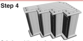
Position the second side panel over the steps and risers and press the panel down so that each step and riser are fully seated into the second side panel. It may be necessary to tap the side panel, using a mallet or a hammer and block of wood, to fully seat it.
