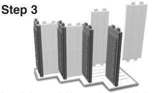
Insert a riser between each of the steps so that the ends of the risers align in the riser recesses on the same panel. Note: Position riser so center hole faces "back" of steps.
