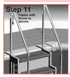
Spray the ends of the handrails with liquid soap or spray lubricant and slip the ends of the handrails into the open ends of the posts until they are fully seated. Secure in place using one #10 x 1-1/4 screw per post.
