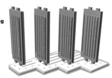
into the openings of the side panel. Make sure that the riser groove in the top of each step is lined up with the riser recess in the side panel and the engraved markings "Danger No Jumping/No Diving" are facing toward the front of the unit.
